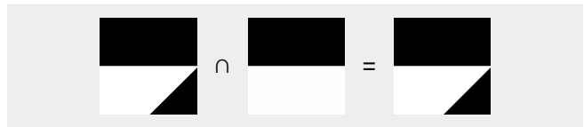
Figure 4: The intersection between the input image and the existing image on the stack to generate a replacement for the image on the stack.
